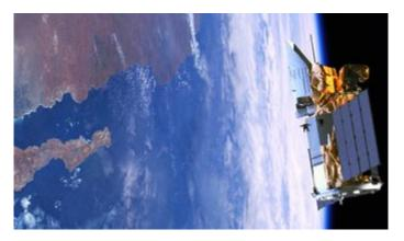
Glory will fly in a low-Earth orbit of 438 miles (705 km) altitude, which is about the distance between Boston and Washington. Photo by NASA
