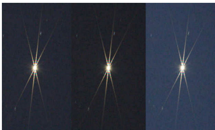
Example diffraction patterns produced by a Bahtinov mask
