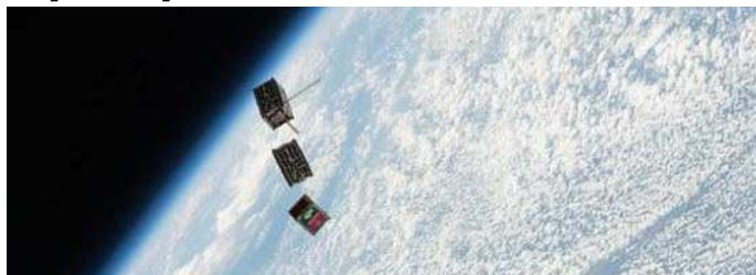
CubeSats being deployed from the International Space Station during Expedition 47. Image: NASA
