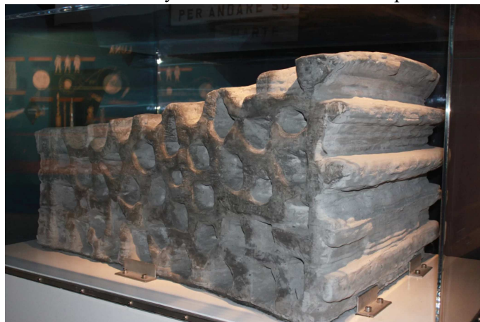
A 1.5 ton building block produced as a 3D-printing demonstration of lunar soil. Credit: ESA
