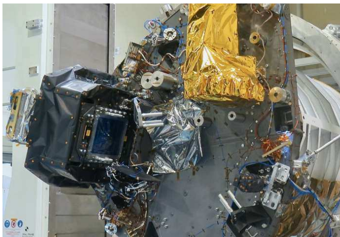
VIS and NISP instruments on Euclid's payload module. Credit: Airbus
