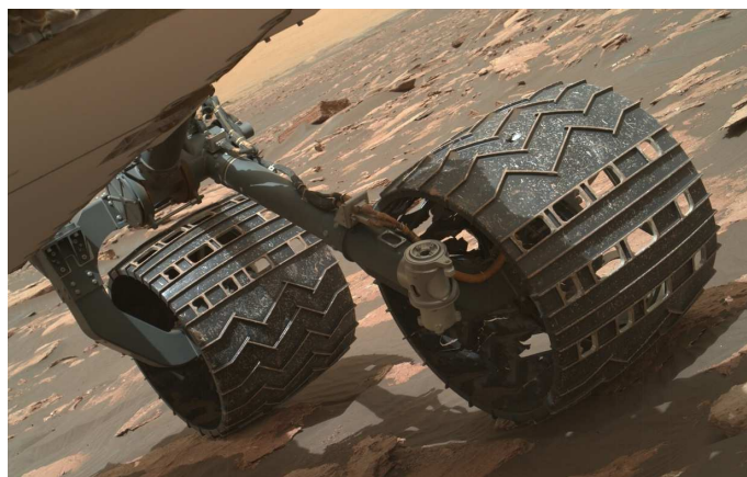
An image showing the odometry features on Curiosity's wheels, taken on Mars on January 26, 2017.
